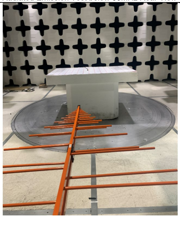
Radiated Emission Test below 1GHz Rear View
