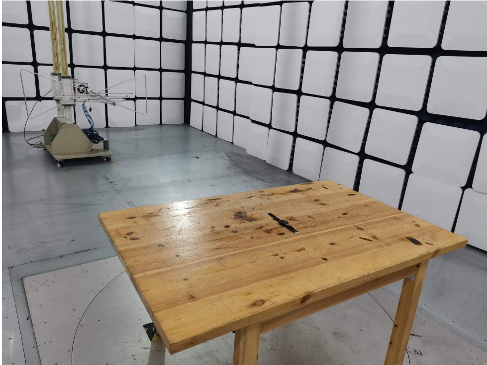
Photo of Radiation Emission Test
