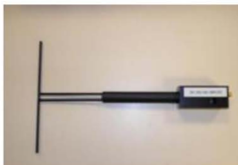
Figure 1 – Satimo COMOSAR Validation Dipole
