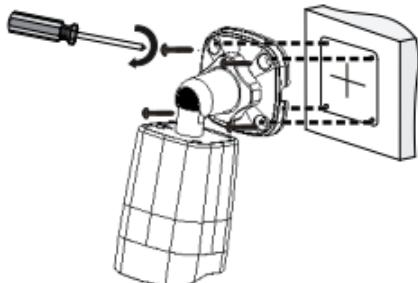
Lead tapping screws through the guide holes in the base and fix them on the wall by using a screwdriver.
