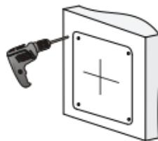
2 Drill 30 mm-depth guide holes according to the positions marked by stickers.
