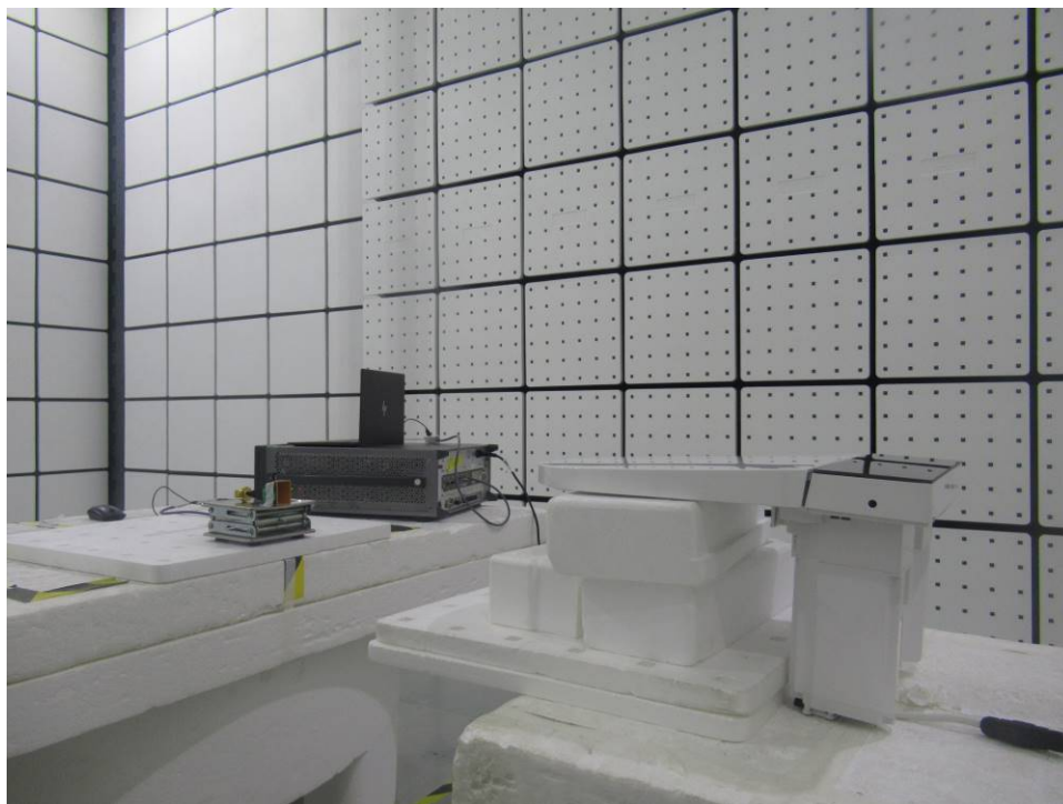
Photograph 5: Set-up photo for Radiated Spurious Emission, 40GHz ~ 50GHz
