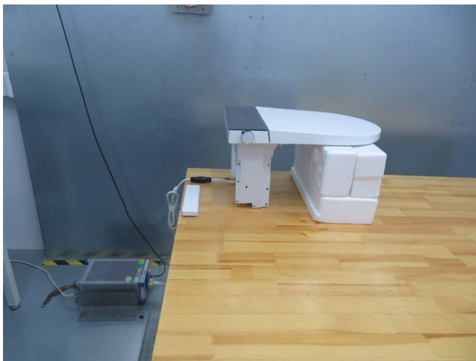
Photograph 8: Set-up photo for Conducted Emission
