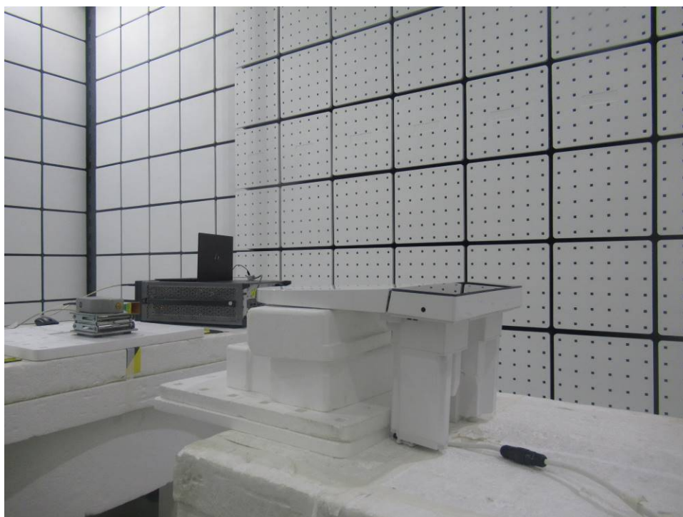
Photograph 6: Set-up photo for Radiated Spurious Emission, 50GHz ~ 75GHz
