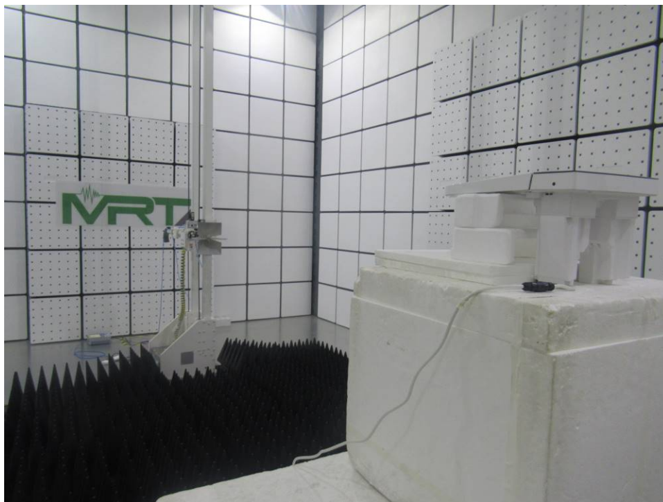
Photograph 3: Set-up photo for Radiated Spurious Emission, 1GHz ~ 18GHz
