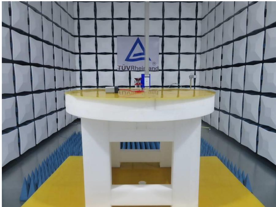
Photograph 2: Set-up photo for Radiated Spurious Emission, 1GHz ~ 18GHz
