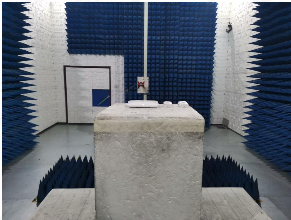
FCC RADIATED EMISSION TEST SETUP ABOVE 1GHZ
