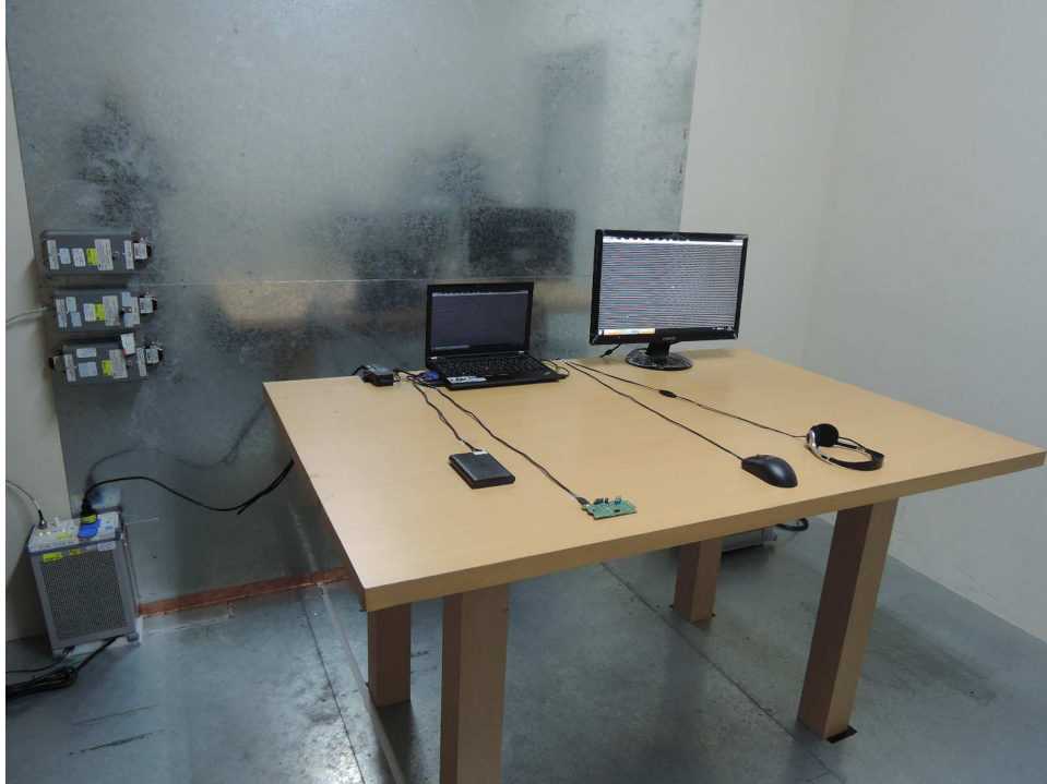
Photograph 6: Set-up for for Mains Conducted testing Front
