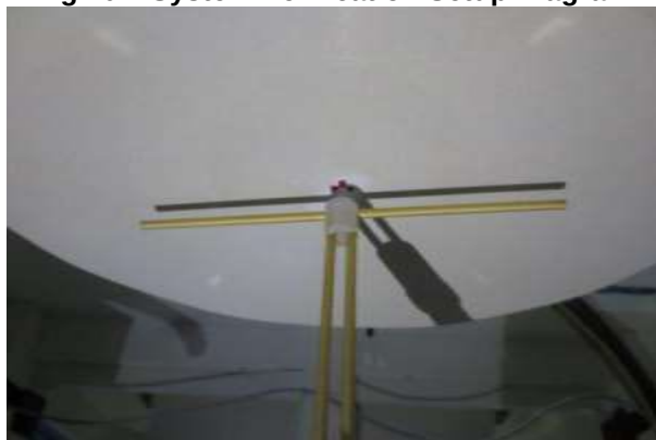
Fig.10.2 Photo of Dipole setup
