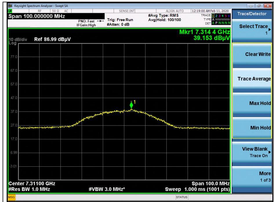
High channel 3<sup>rd</sup> harmonic (Peak)
