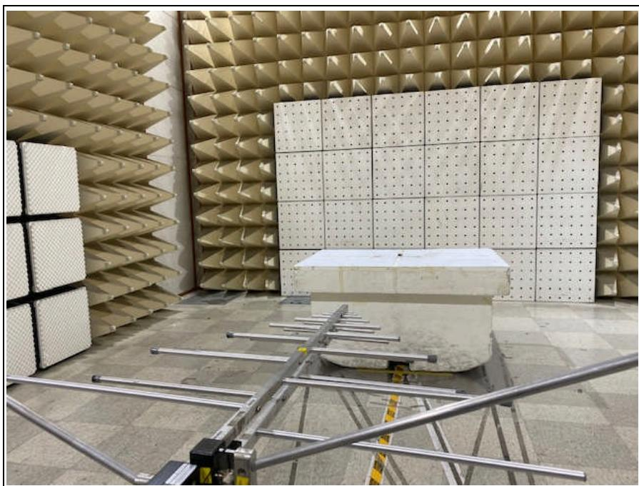
**3. Photo of Radiated Spurious Emission Test (Above 1 GHz)**
