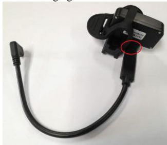
Figure 3. Connect thermal imaging module to connector
