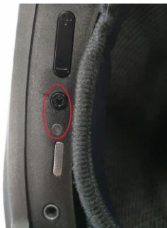
Figure 9. Schematic diagram of power switch position
