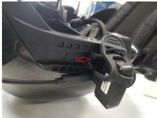
Figure 4. Install the thermal imaging module on the guide rail
