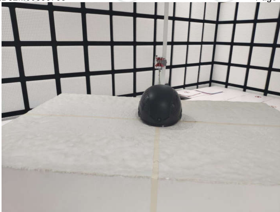
Radiated spurious emission Test Setup-3(Above 1GHz)
