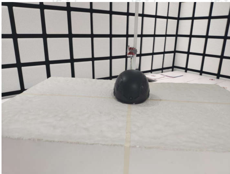
Radiated spurious emission Test Setup-3(Above 1GHz)
