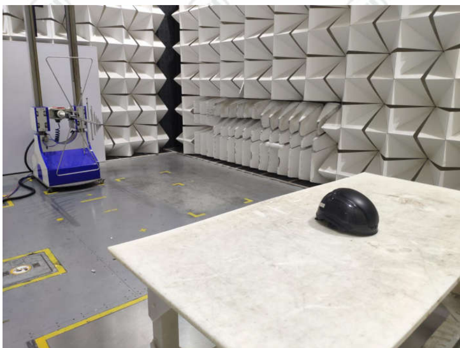
Radiated spurious emission Test Setup-2(Below 1GHz)
