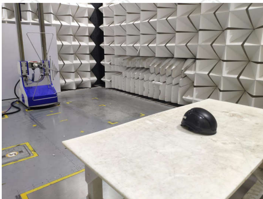
Radiated spurious emission Test Setup-2(Below 1GHz)
