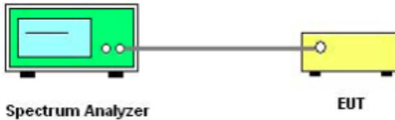
The EUT is connected to the Spectrum Analyzer; the RF load attached to the EUT antenna terminal is 50Ω; the path loss as the factor is calibrated to correct the reading. Make the measurement with the spectrum analyzer's resolution bandwidth (RBW) = 100 kHz. In order to make an accurate measurement, set the span greater than RBW.
