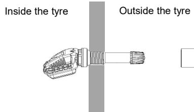
1.4 Place nut<sup>④</sup> on the valve stem, and tighten with 5 Nm (44 inch pounds) torque.
