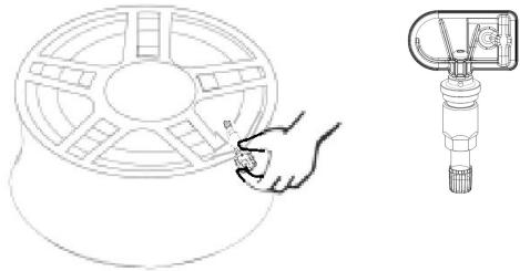
1.3 Take off the nut<sup>④</sup>, insert the valve stem through the rim hole from inside.
