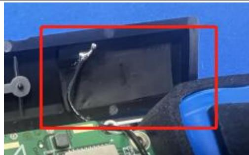
The antenna is FPC antenna with ipex connector. The best case gain of the 5G WiFi antenna is 1.73dBi@5GHz: Wi-Fi: U-NII-1, 3.43dBi@5GHz: Wi-Fi: U-NII-3
