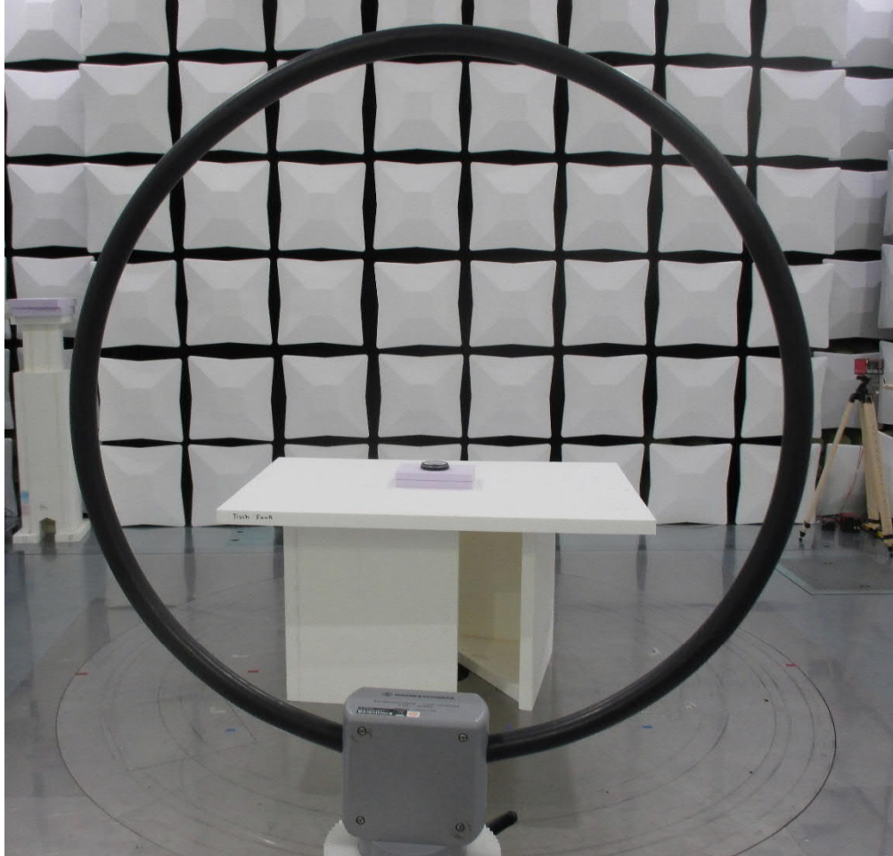
Test setup semi anechoic chamber TX spurious emissions from 9 kHz to 30 MHz
