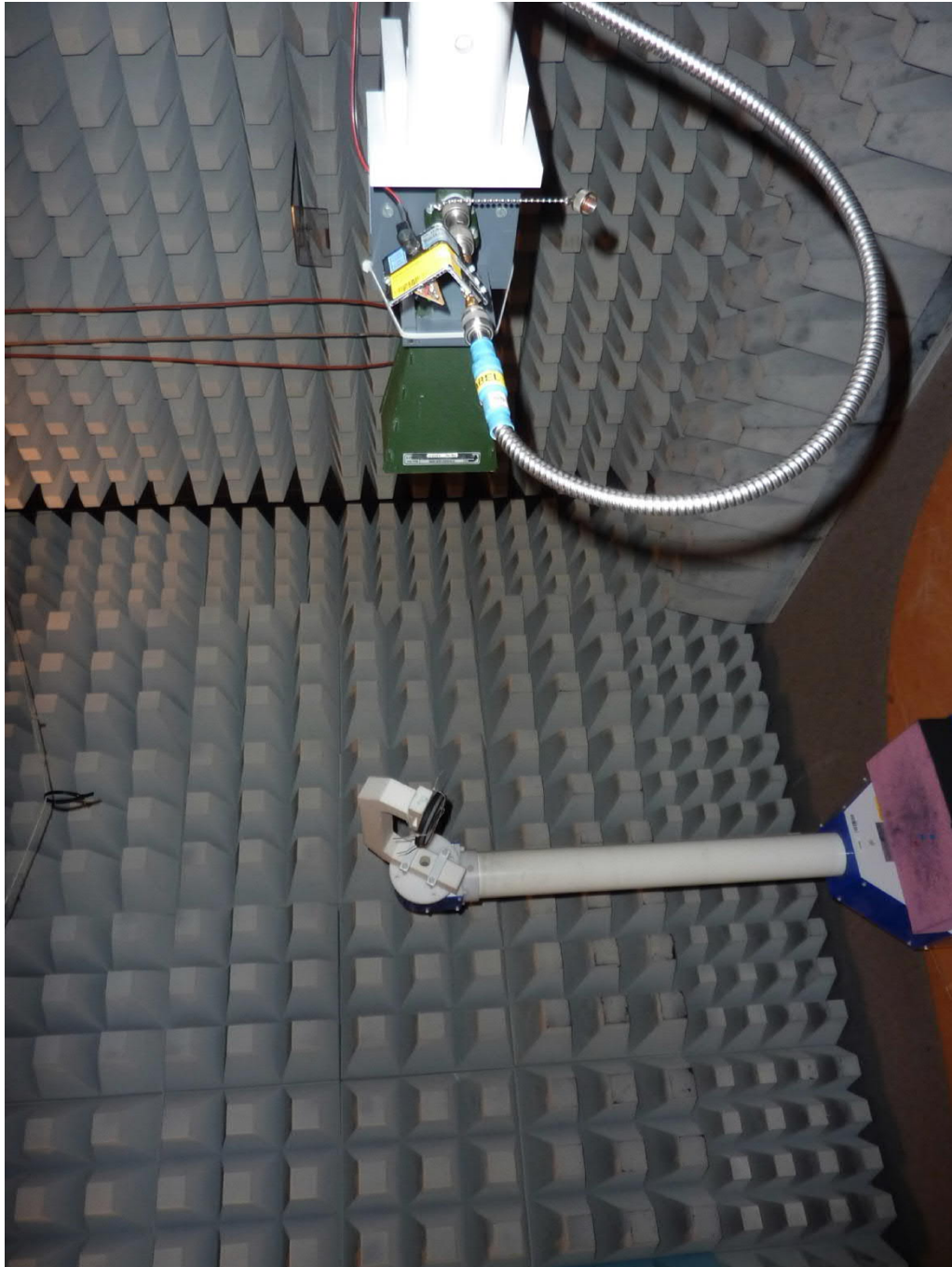
Test setup fully anechoic chamber TX spurious emissions from 3.1 GHz to 10.6 GHz
