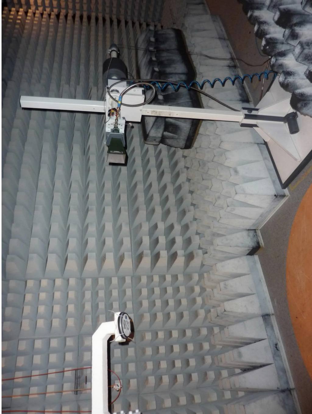
Test setup fully anechoic chamber TX spurious emissions from 1 GHz to 40 GHz
