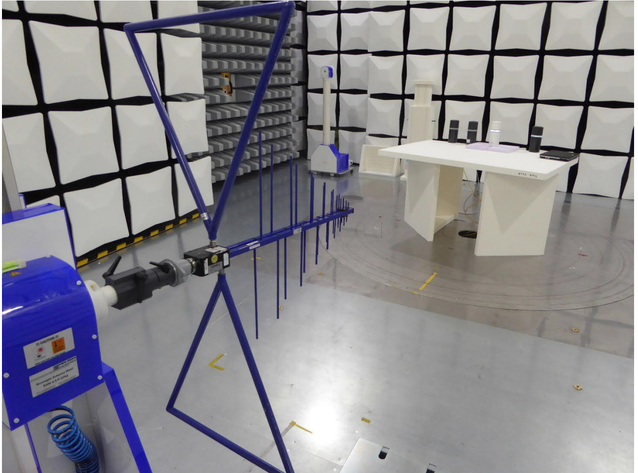
Test setup semi anechoic chamber TX spurious emissions from 30 MHz to 1 GHz
