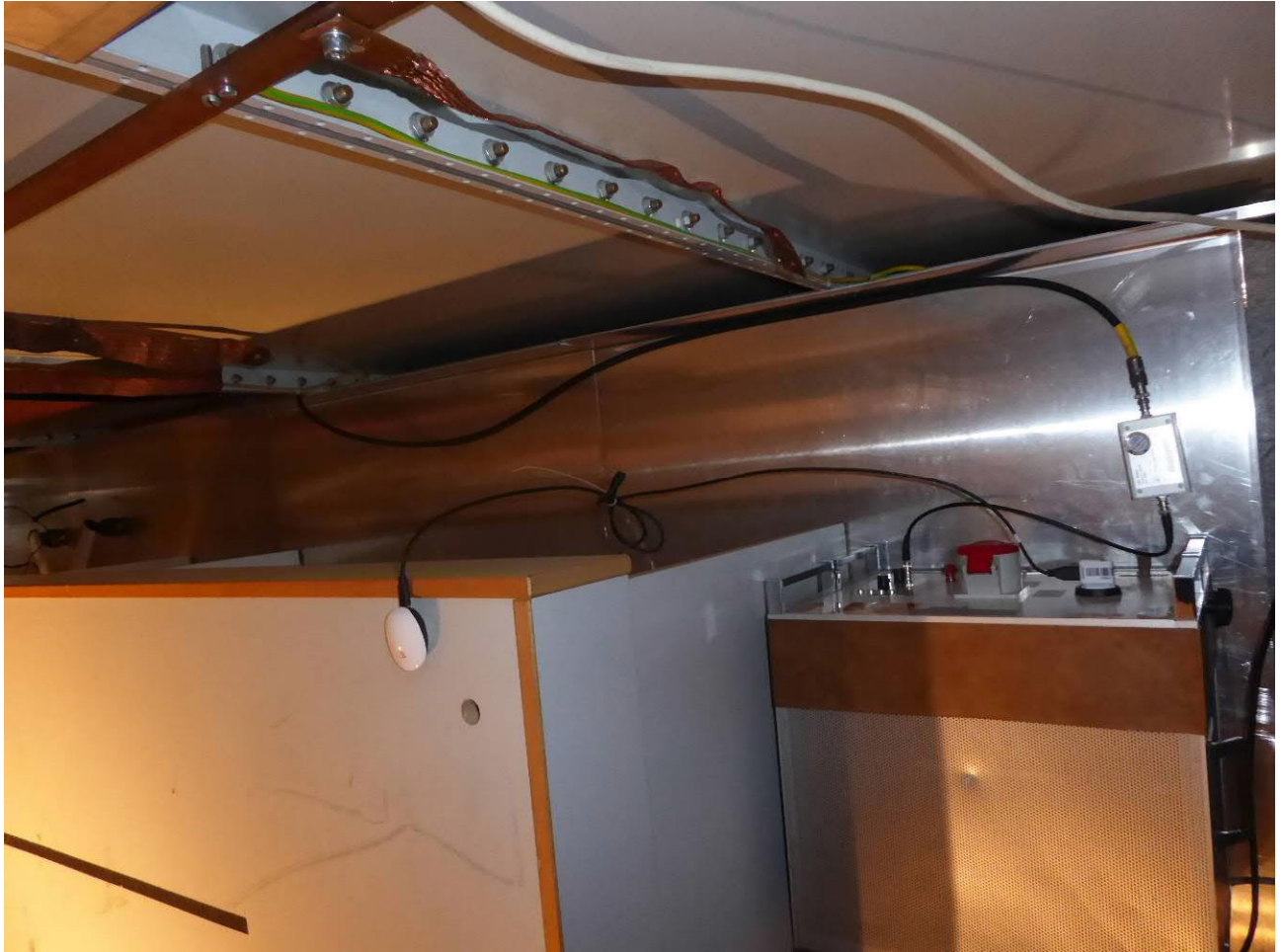
Test setup SmartAntenna – conducted emissions on power supply lines
