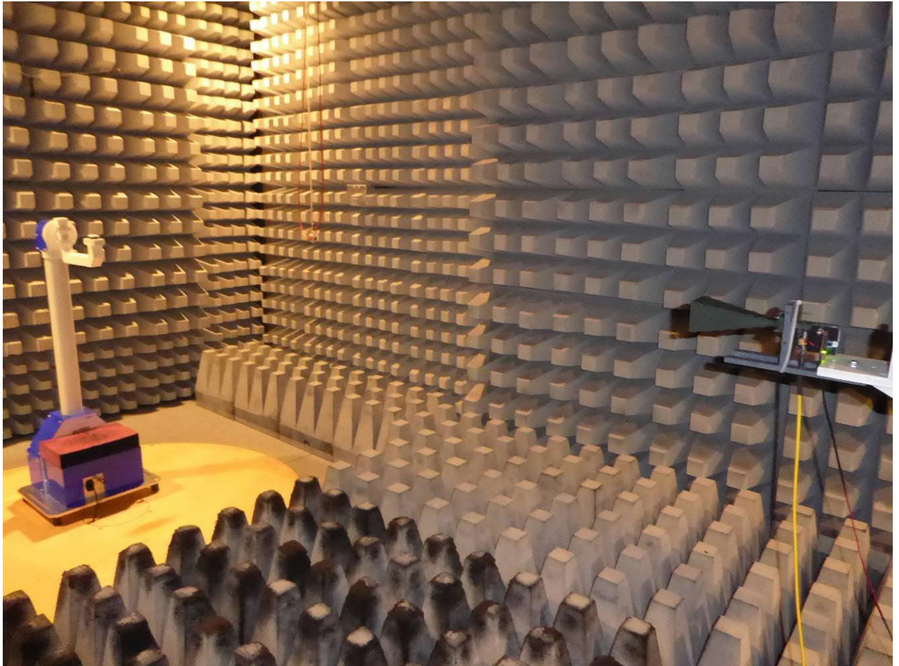
Test setup WTag – radiated test in anechoic chamber (M20)
