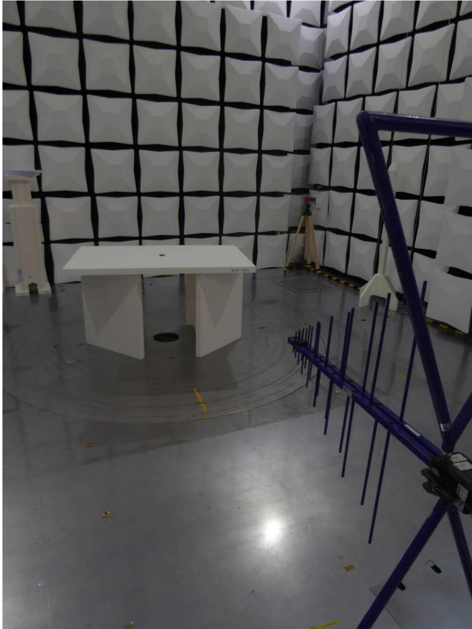
Test setup WTag – radiated test in anechoic chamber (M276)
