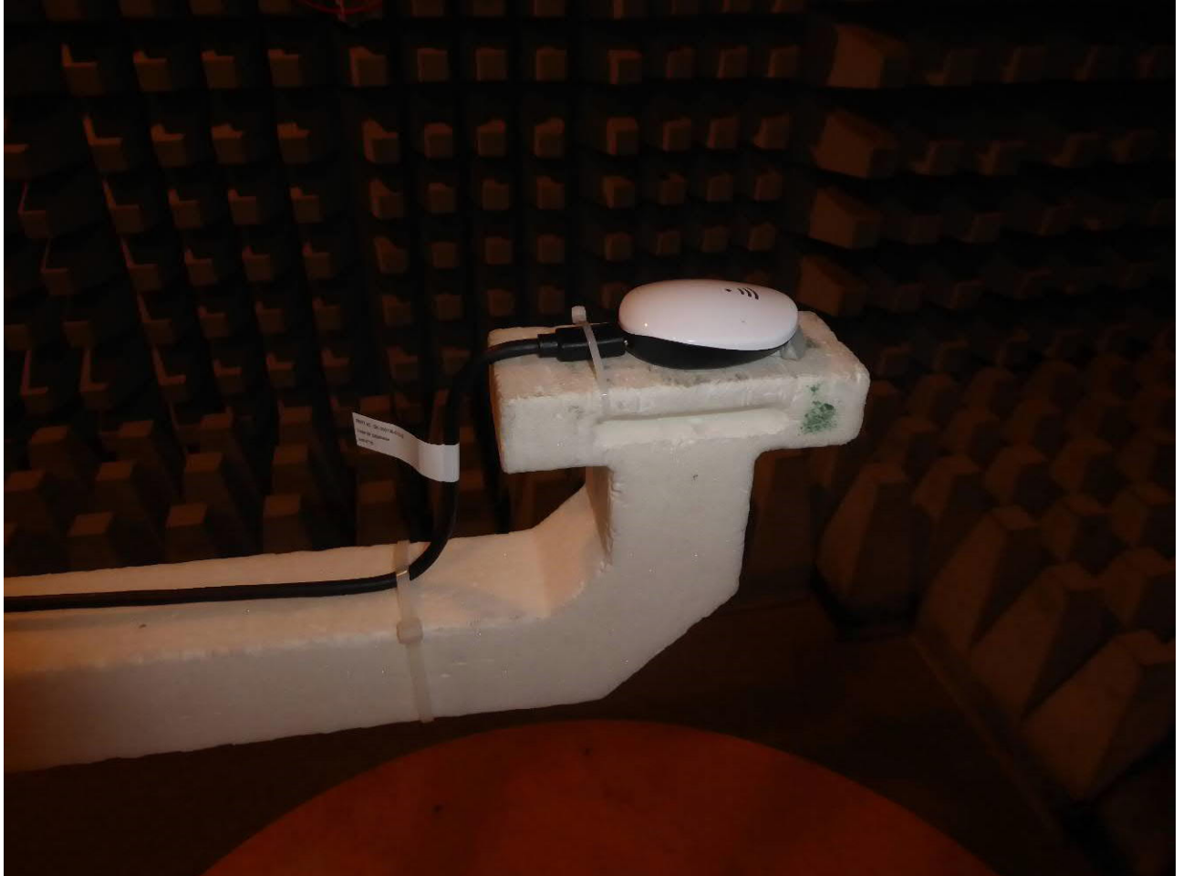
Test setup SmartAntenna – radiated test in anechoic chamber (M20)
