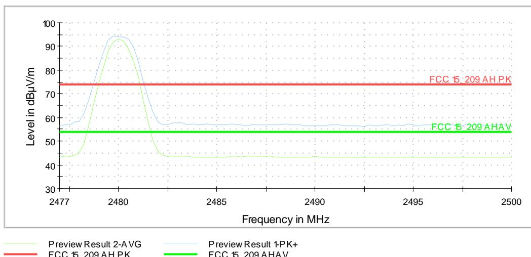
Transmitter operates at the lower end of the assigned frequency band (operation mode 1)
