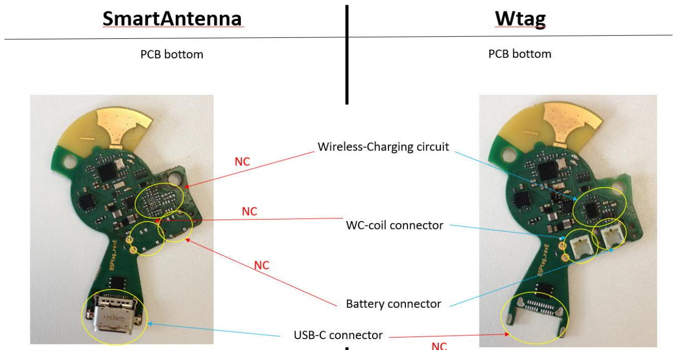
The test modes at the SmartAntenna EUT were set using a USB cable connected to a laptop PC. Using a terminal program, the test modes were set for the tests.
