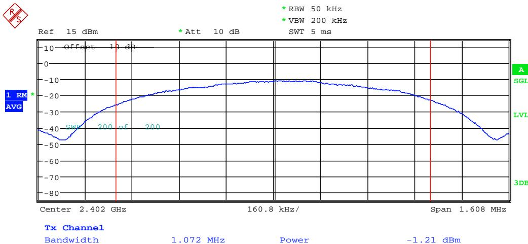
The antenna gain is below 6 dBi, therefore no conducted output limit reduction is necessary.
