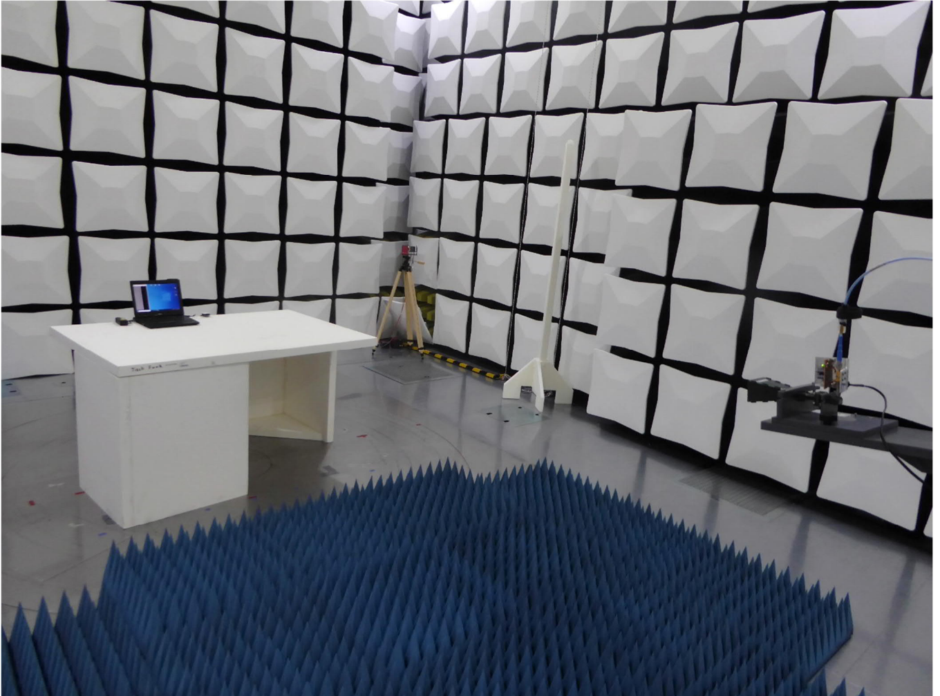
Test setup SAC with floor absorbers radiated emission 18 – 26.5 GHz
