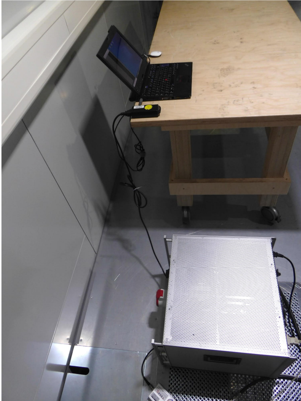
Test setup power line conducted
