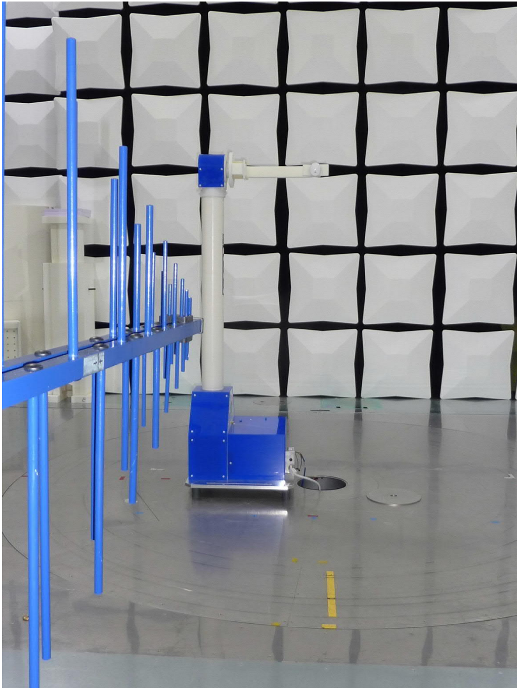
Test setup semi anechoic chamber spurious emissions from 30 MHz to 1 GHz
