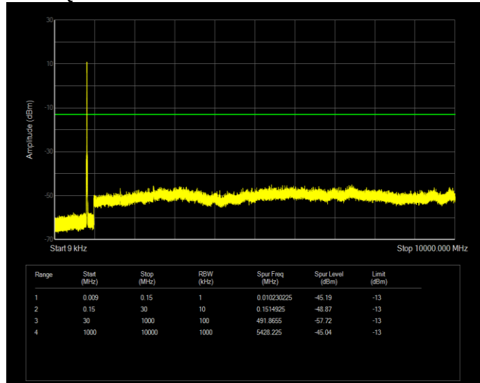
Band5 QPSK BW=10MHz Channel=20525 RB Size=50 Position=#0
