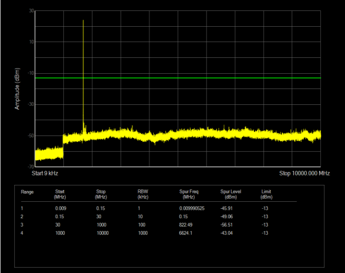
Band4 QAM16 BW=1.4MHz Channel=19957 RB Size=6 Position=#0
