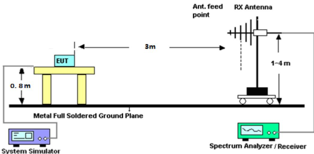
For radiated test from above 1GHz
