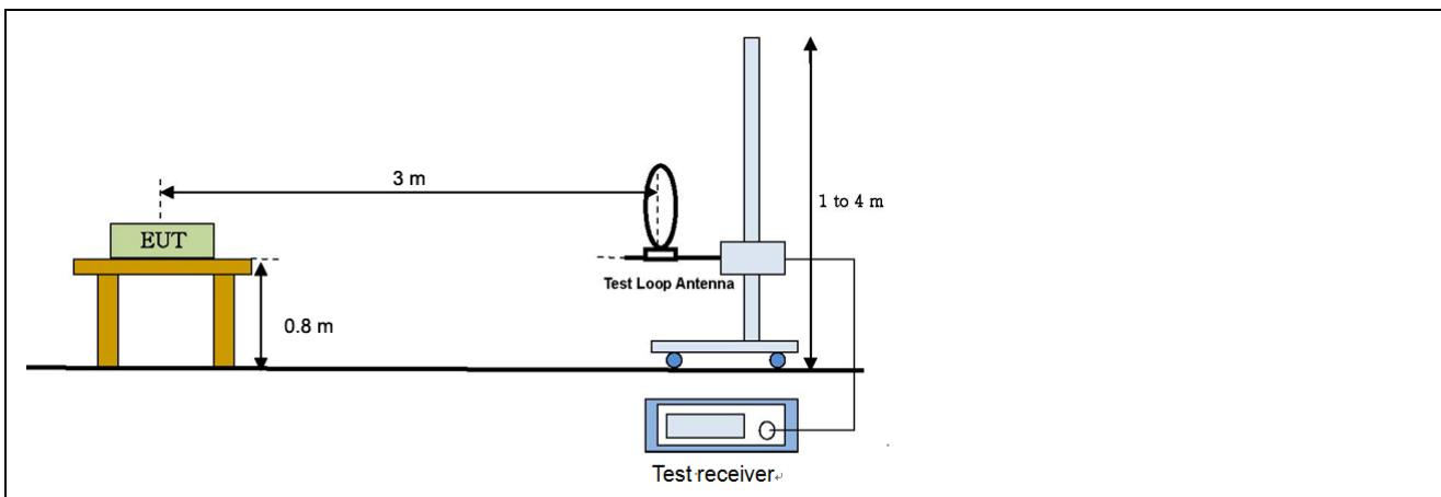
Radiated emission setup, Below 1 000 MHz
