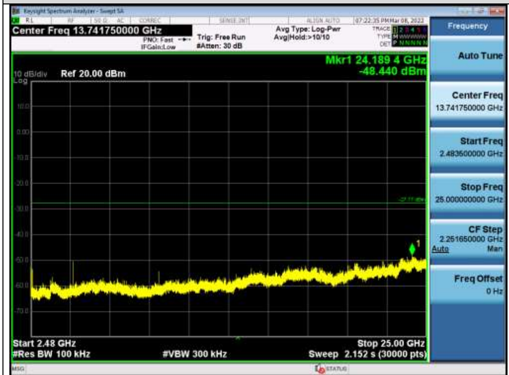
Test_Graph_BR_ANT1_2441_1Mbps_Higher Band Emissions
