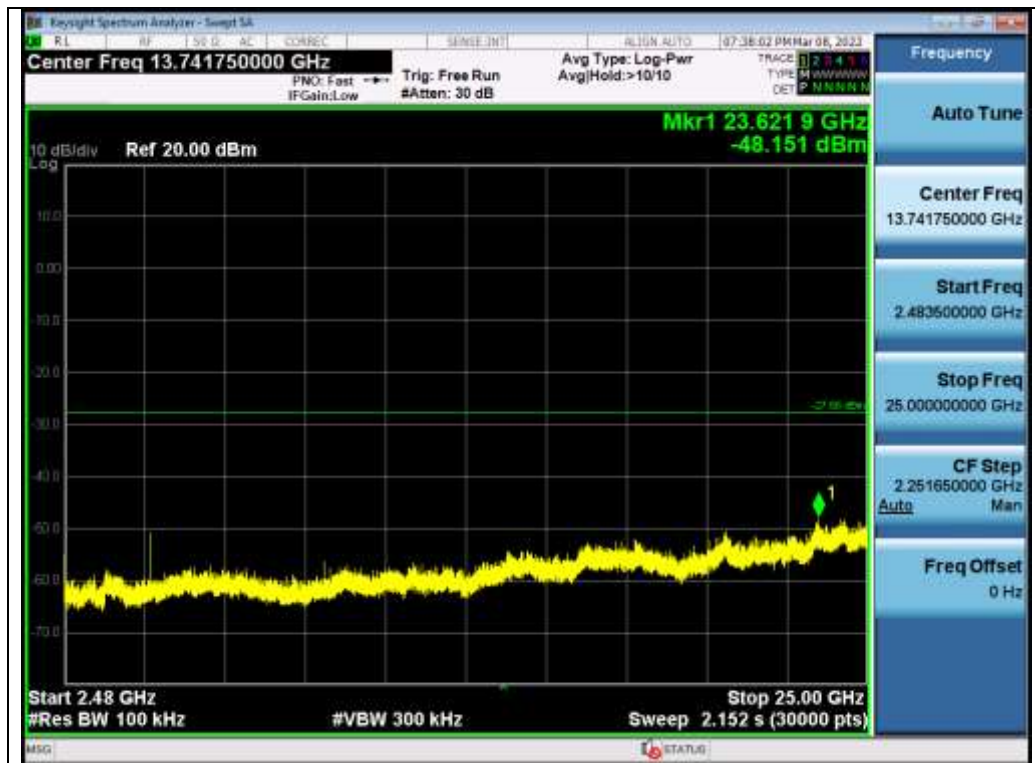
Test_Graph_EDR_ANT1_2441_2Mbps_Higher Band Emissions
