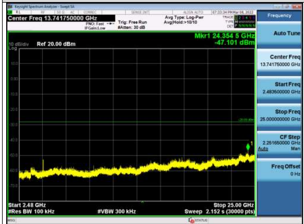
Test_Graph_EDR_ANT1_2402_2Mbps_Higher Band Emissions
