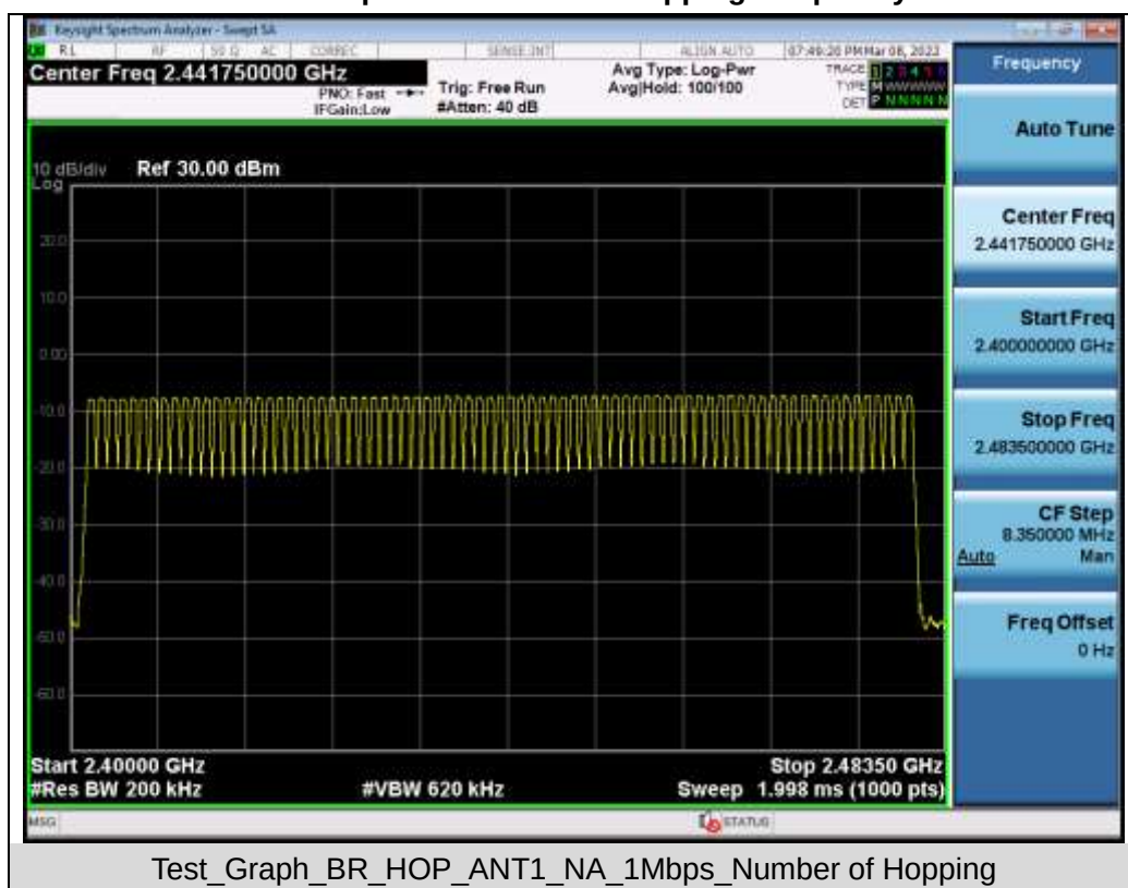
Test Graphs of Number of Hopping Frequency
