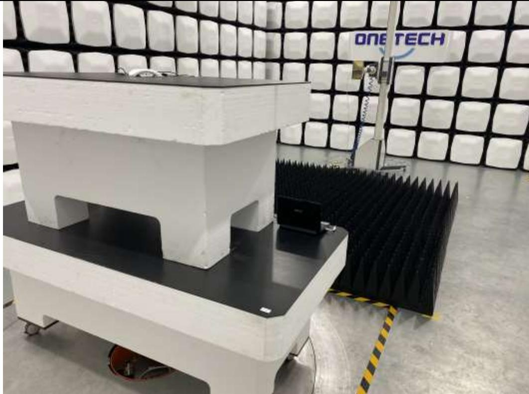
**[WLAN 2.4 GHz]****- Conducted Emission Test**
