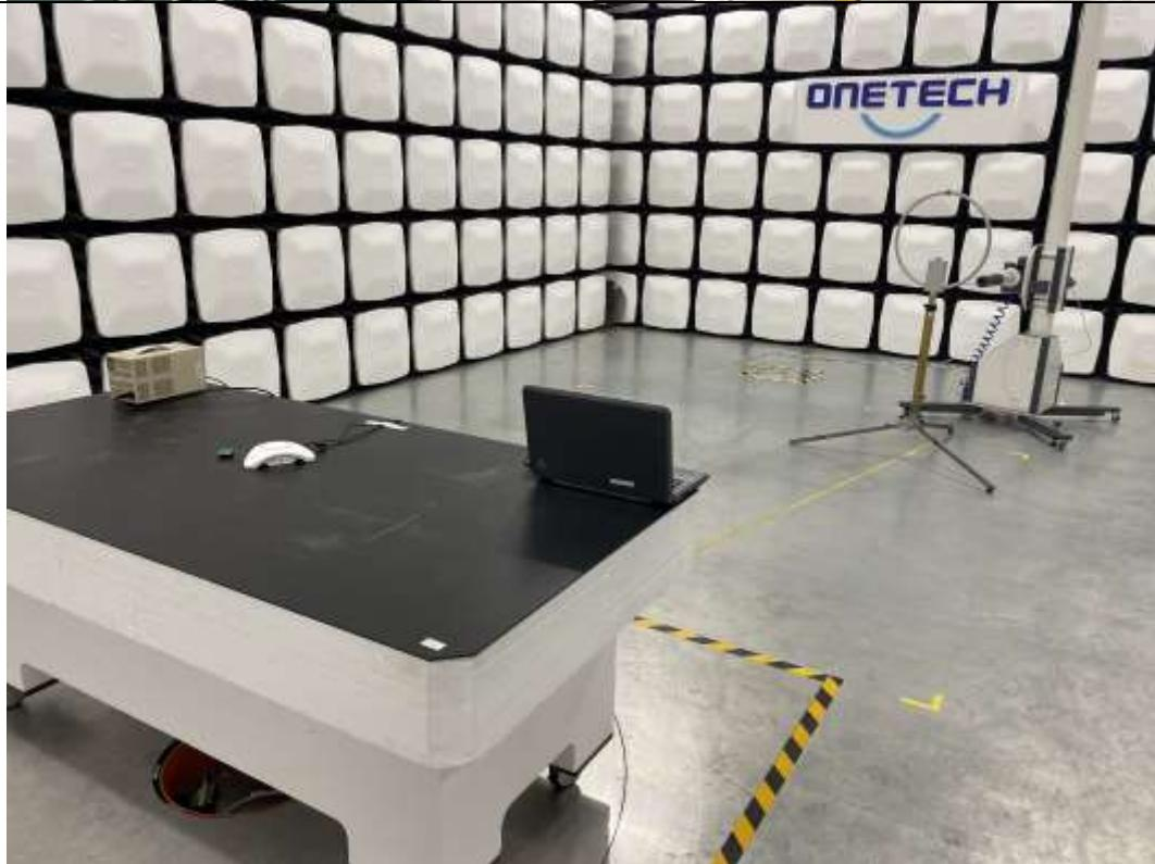
**- Radiated Emission Test (Below 1 GHz)**
