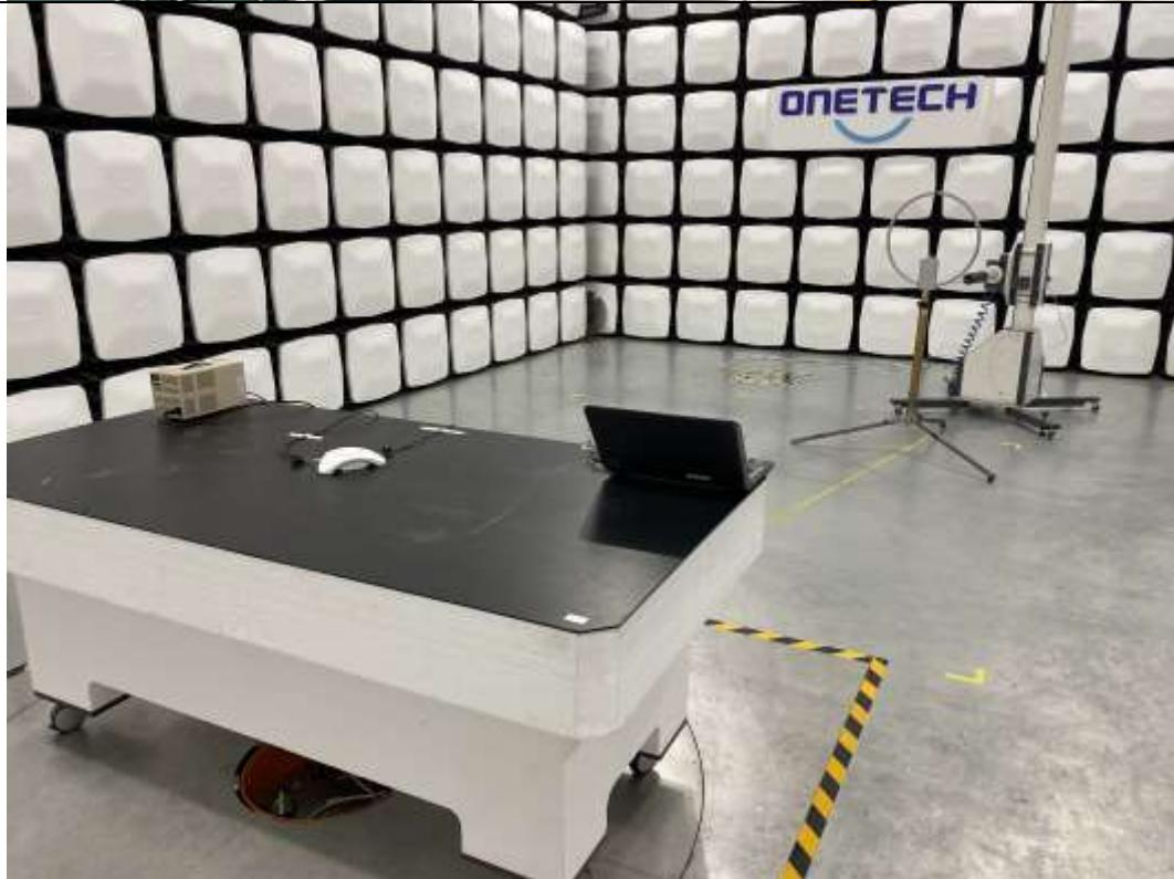
**- Radiated Emission Test (Below 1 GHz)**
