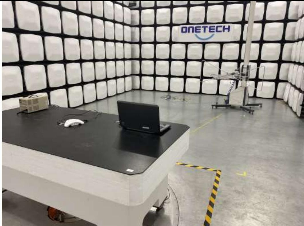
**- Radiated Emission Test (Above 1 GHz)**
