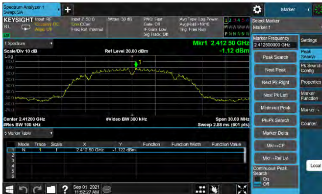
802.11b LOW CHANNEL, Carrier level
