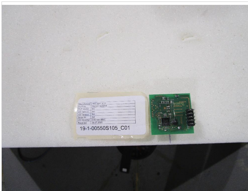
Photograph 4: EUT Setup Magnetic Field Measurements in the Semi anechoic chamber
