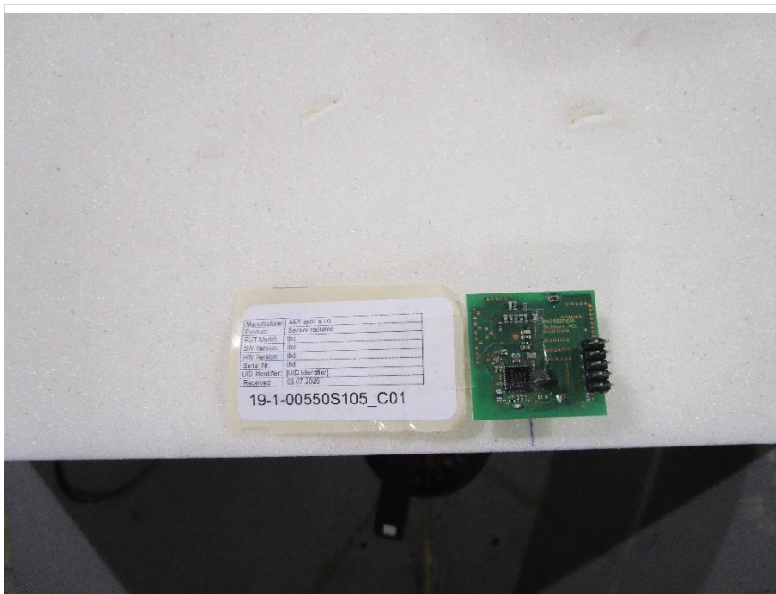
Photograph 6: EUT Setup Electrical Field Measurements in the Semi anechoic chamber
