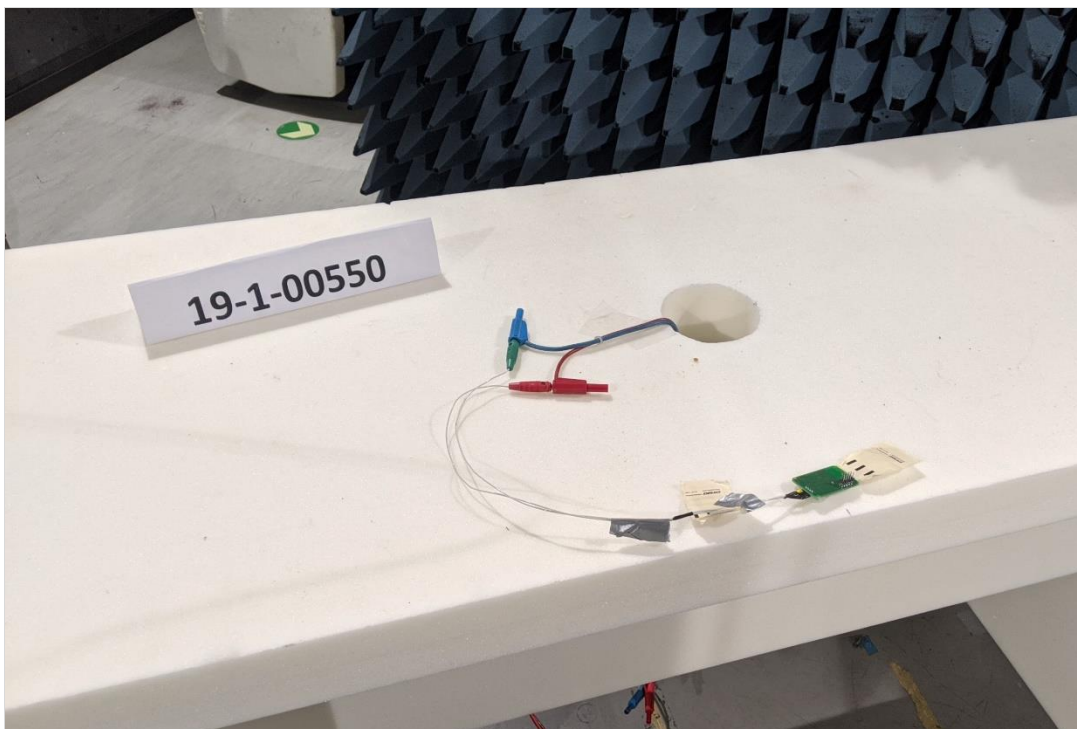
Photograph 4: EUT Test Setup in the semi anechoic chamber, Radiated interference field strength
