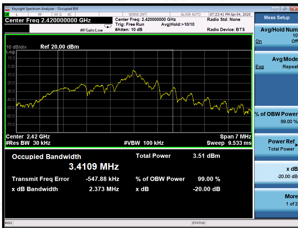
TEST PLOT OF BANDWIDTH FOR LOW CHANNEL
