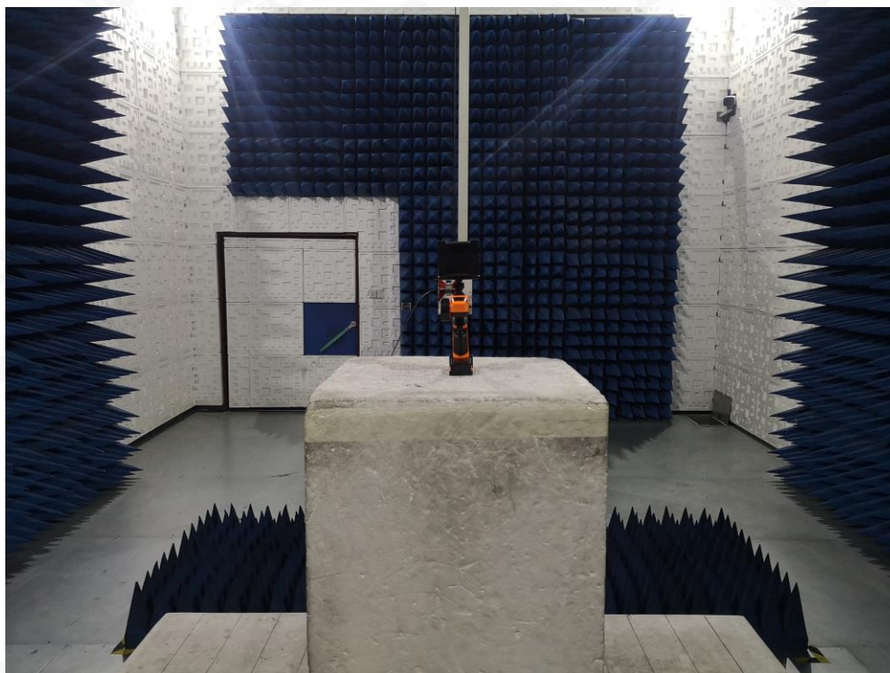
FCC RADIATED EMISSION TEST SETUP ABOVE 1GHZ
