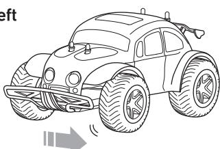
If the car tends to drift to the left, move the trimmer (beneath the car) to the left to adjust the steering.
