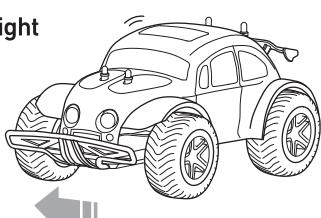
If the car tends to drift to the right, move the trimmer (beneath the car) to the right to adjust the steering.
