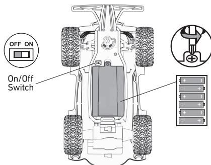
III Open battery cover and install 1 9V battery (included). Replace the cover.
