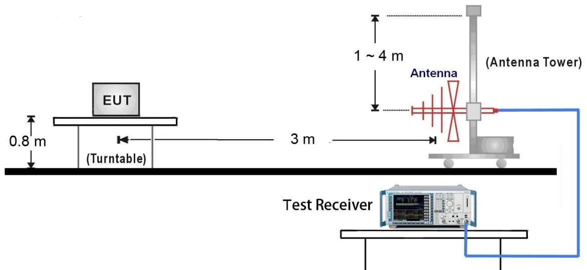
1GHz ~ 18GHz Test Setup:
