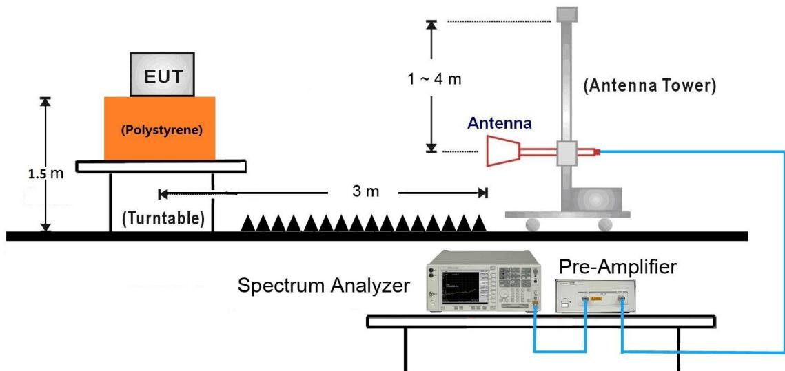
18GHz ~25GHz Test Setup:
