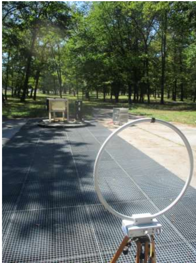
Figure 2: Radiated emission test 9 kHz – 30 MHz: measurement in OATS with 10 m measurement distance
