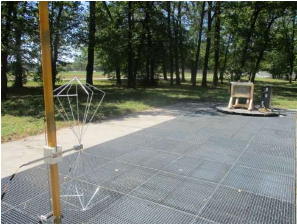
Figure 4: Radiated emission test 30 MHz – 200 MHz: measurement in OATS with 10 m measurement distance
