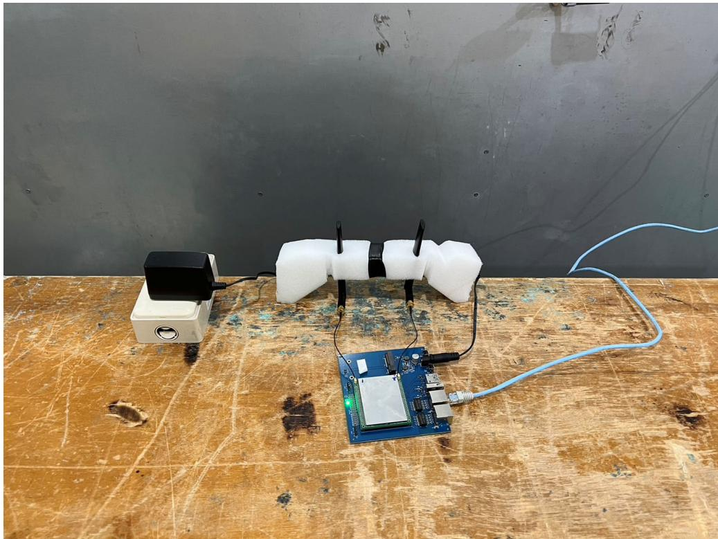
Radiated Emission Set up Photos
