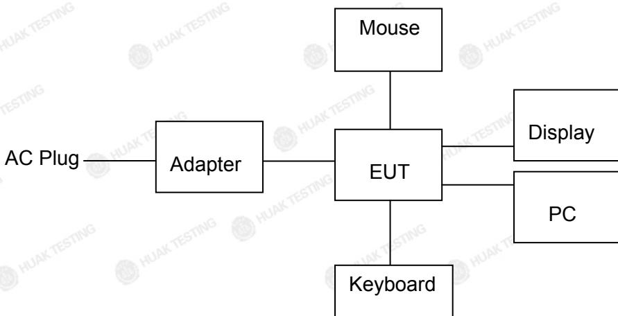
Operation of EUT during radiation above 1GHz testing:
