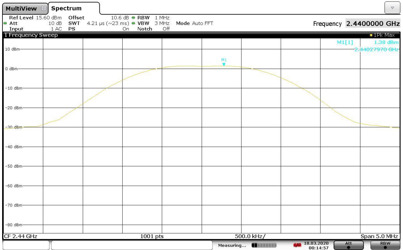
Figure 2 – Output Power CH19 2440 MHz
