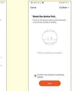
5.Gateway power on,long press the setting button on the gateway until the red indicator light flash quickly and blue light is on for long. Click "Confirm" the indicator is
