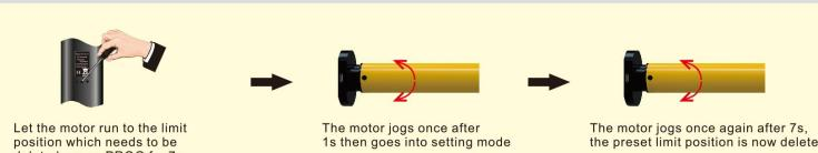
Let the motor run to the limit position which needs to be deleted, press PROG for 7s
