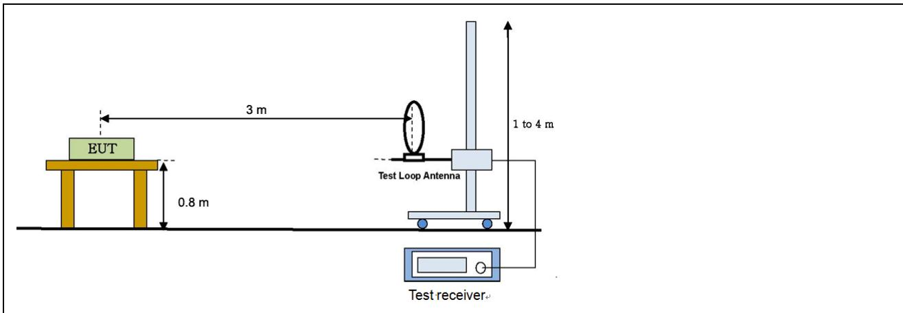
Radiated emission setup, Below 1 000 MHz
