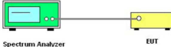
The EUT which is powered by the Battery, is connected to the Spectrum Analyzer; the RF load attached to the EUT antenna terminal is 50 Ohm; the path loss as the factor is calibrated to correct the reading. Make the measurement with the spectrum analyzer's resolution bandwidth(RBW) = 100 kHz. In order to make an accurate measurement, set the span greater than RBW.
