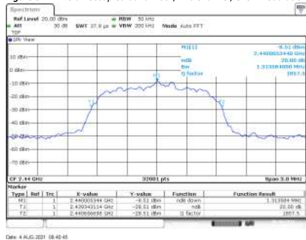
Figure 8.2-6: 20 dB occupied bandwidth, Mid channel, 8-DPSK modulation
