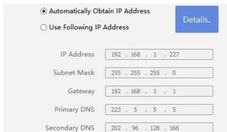
\*This user manual takes LAN port as an example. After connecting the Ethernet cable, the player automatically gets the IP address. Once configured, program editing, program publishing, and device management are available through LAN.
