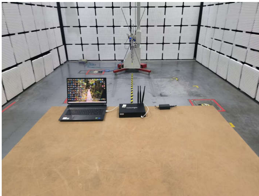
Radiated spurious emission Test Setup-1(Below 1GHz)
