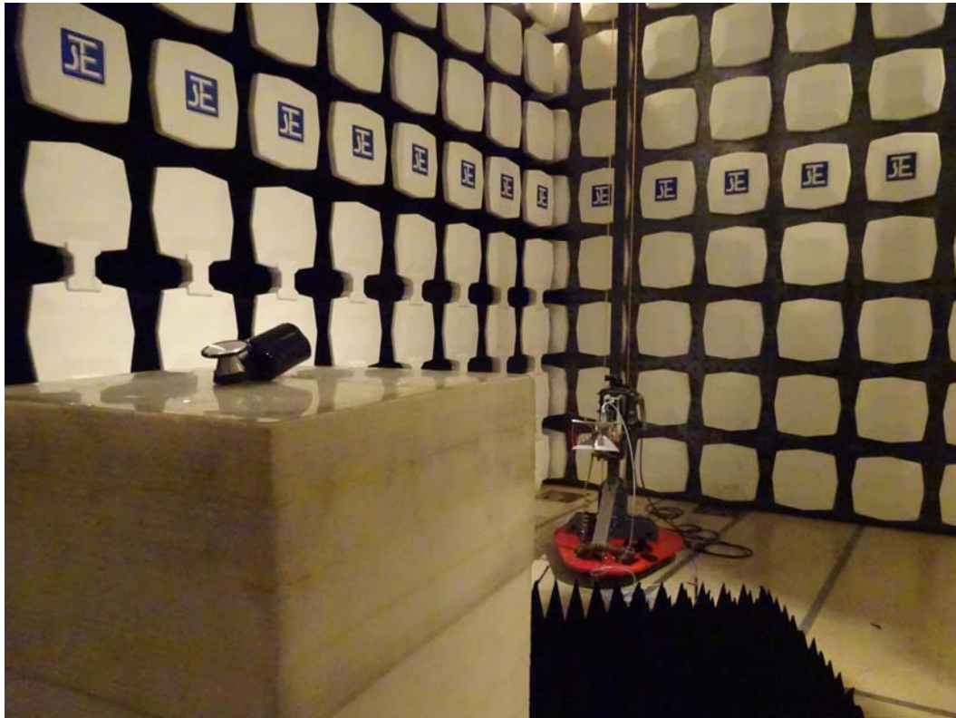
Measurement of Radiated Emission Test Set Up
