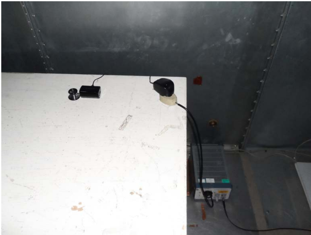
Measurement of Conducted Emission Test Set Up
