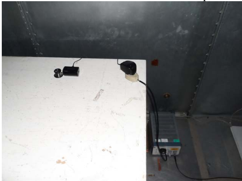
Measurement of Conducted Emission Test Set Up
