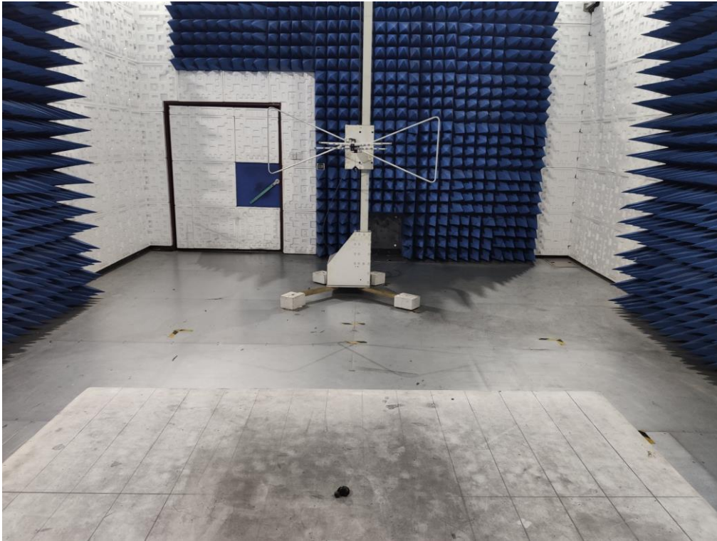
RADIATED EMISSION TEST SETUP ABOVE 1GHZ
